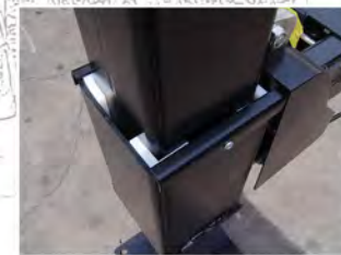
Exclusive wrap-around crossbar design. Box steel leg surrounded by an exterior steel sleeve ensures positive contact
